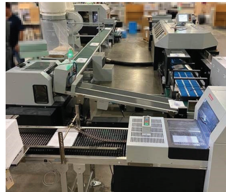
The Horizon SB-09V Perfect Binder runs inline with the HT-1000V Three-knife Trimmer at 3,000 books per hour to seamlessly handle the increased volume required by KP's client.
