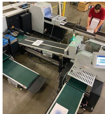
The Horizon SB-09V Perfect Binder runs inline with the HT-1000V Three-knife Trimmer at 3,000 books per hour to seamlessly handle the increased volume required by KP's client.
